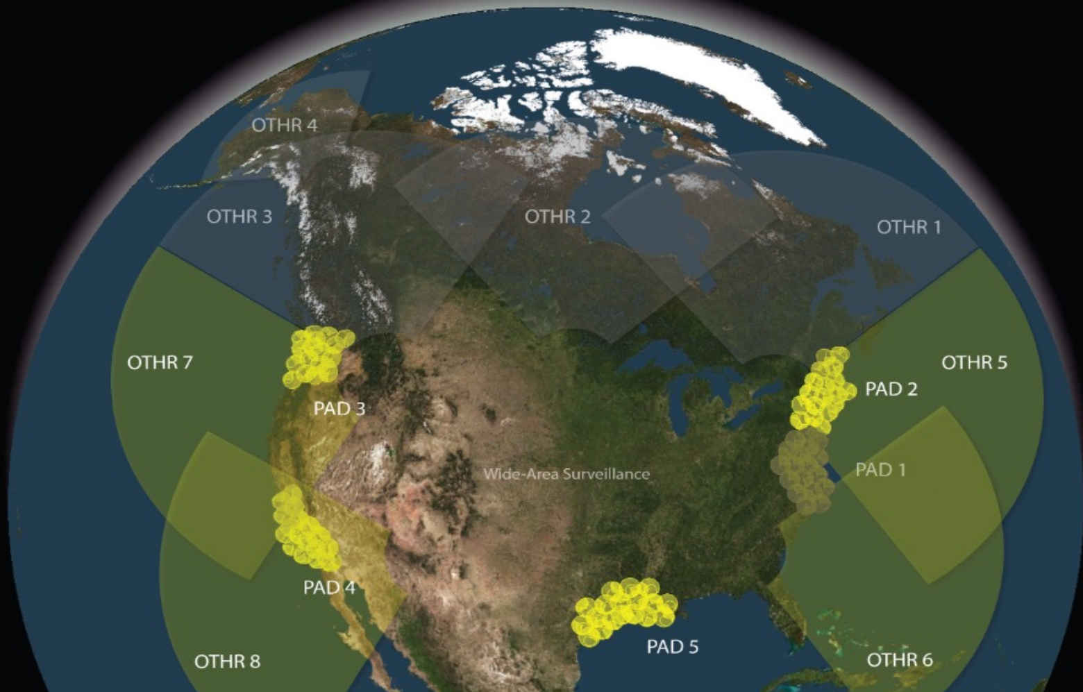
Figure 5: Conception of Homeland Cruise Missile Defense. Source: Center for Strategic and International Studies. PAD = Prioritized area defenses (includes medium-range surface-to-air interceptors and a second interceptor layer with Aegis-type interceptors, linked to sensor towers and other available sensors). OTHR = Over the horizon radar.
