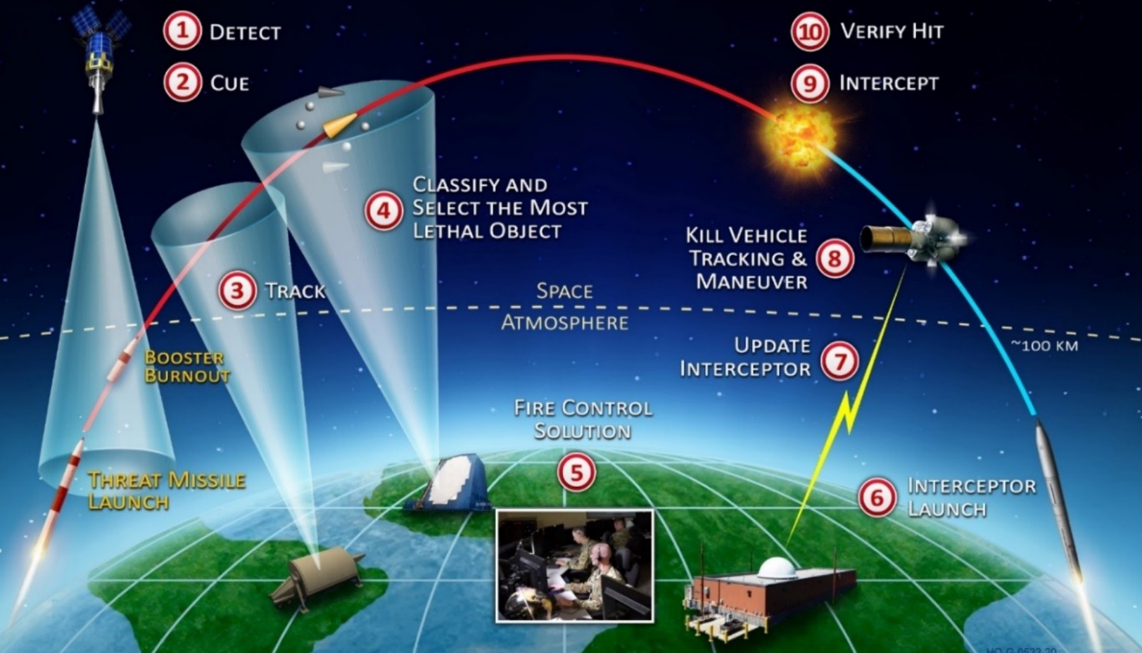
Figure 2: Ten Steps of a Successful Ballistic Missile Intercept. Source: Courtesy US Missile Defense Agency, overview briefing, October 2023.
