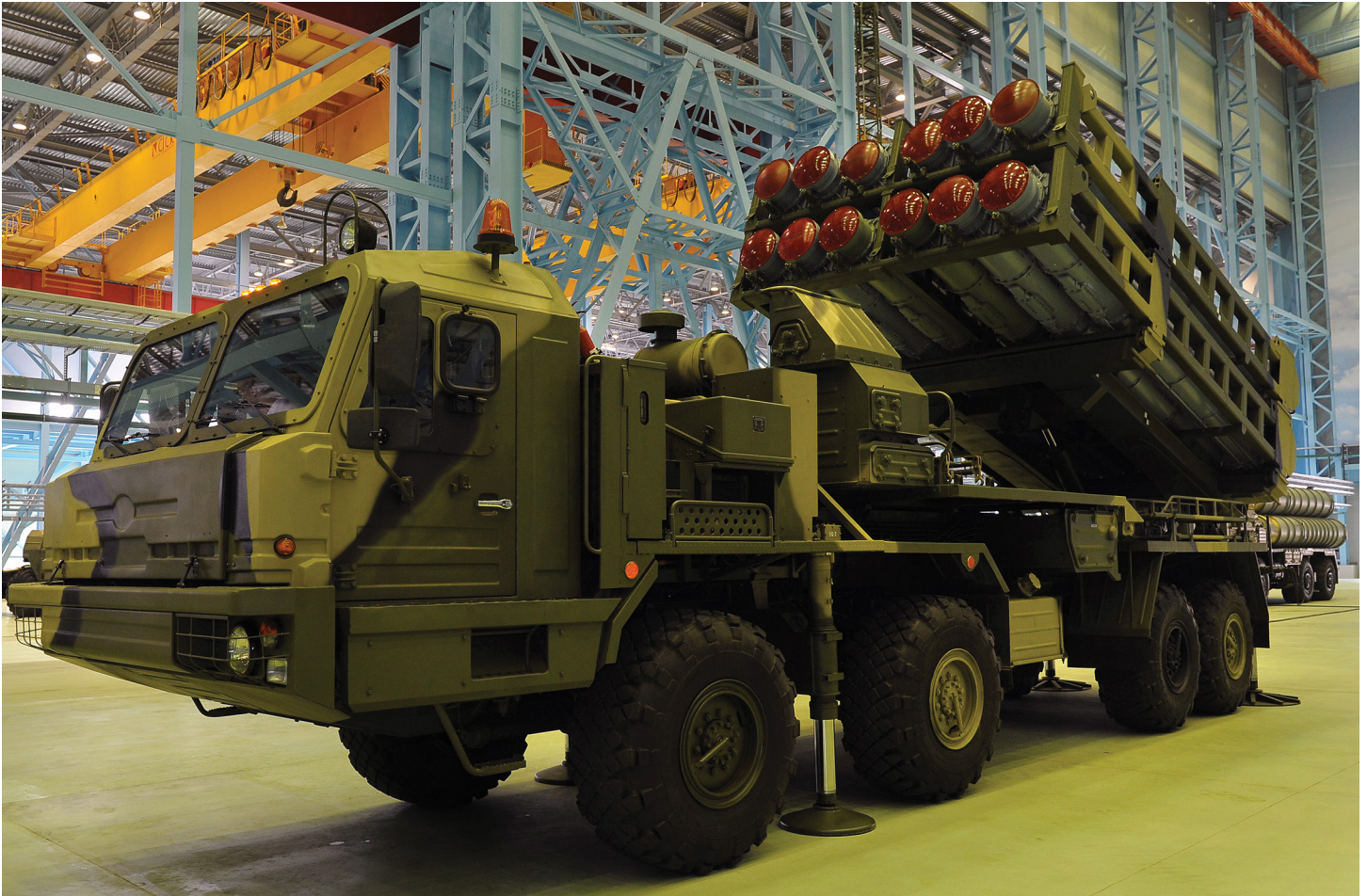
A Russian 50P6 missile launcher of the S-350 which was created to replace the S-300PS variant of the S-300 missile defense system. Source: Wikimedia user Zumlik
