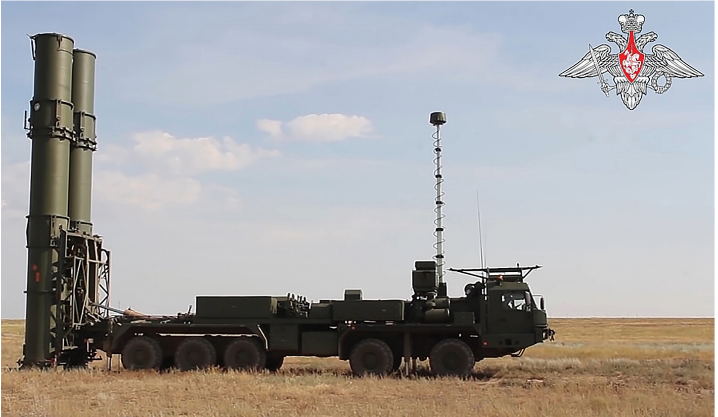
A mobile launch vehicle of Russia's new S-500 air defense system. Source: Russian Ministry of Defense
