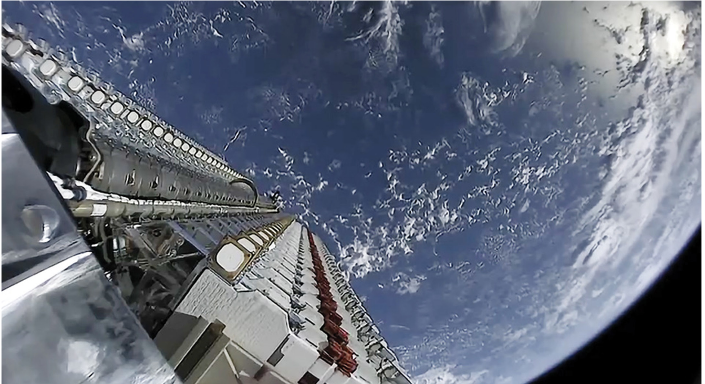
A batch of 60 Starlink test satellites stacked atop a Falcon 9 rocket to be put in orbit. Source: SpaceX, Wikimedia Commons, May 24, 2019, https://commons.wikimedia.org/wiki/File:Starlink_Mission_(47926144123).jpg
